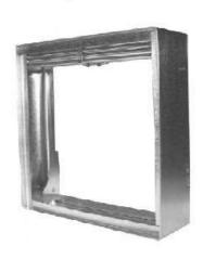
Riyadh seasons manufactures Fire Dampers, which are designed to stop the spread of fire by means localizing areas of fire zones to prevent the distribution of fire through air conditioning duct or wall in central HVAC systems. These fire dampers offer and effective fire barrier by maintaining integrity in a fire situation And are rated up to two to four hours rating, combined with low leakage characteristics.
