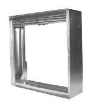
Blade edge seals are silicon edge type, mechanically locked into blade edges. Jamb seals are flexible stainless steel sheet compression type to further ensure low leakage of air/smoke .it is 3 hour fire rating and classification leakage as well .classification (air/smoke leakage shall be not greater than 10 CFM/Ft2 at pressure difference 1"in wg, or 20 CFM/Ft2 at pressure deference 4"in wg.)
