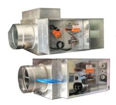
Bypass terminal units handle constant supply of primary air through its inlet and uses a diverting damper to bypass part of supply air into the plenum return. The damper is directly controlled by a room thermostat on the occupied space to provide the volume of air required to meet the thermal demand. The pressure requirement through the supply air path to the conditioned space is set with an inlet balancing damper.
